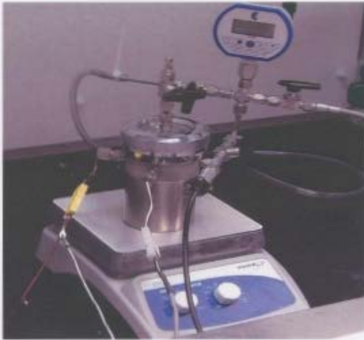
Figure 46 The picture of ARSST™ standard containment vessel
