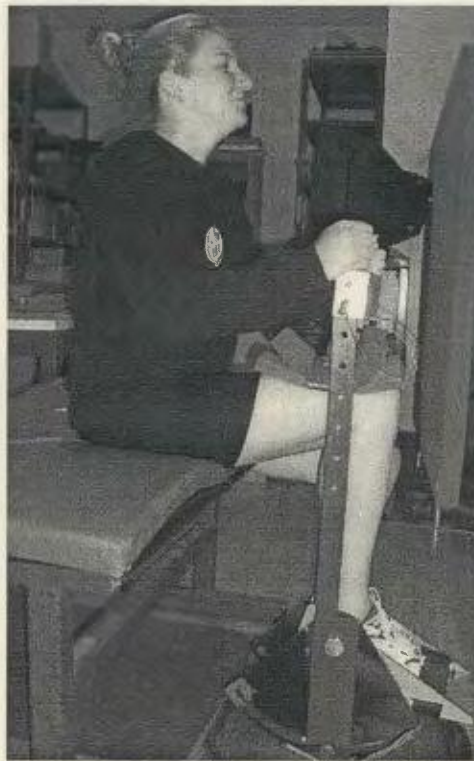
Figure 3 Plantar Flexor MVC set-up
