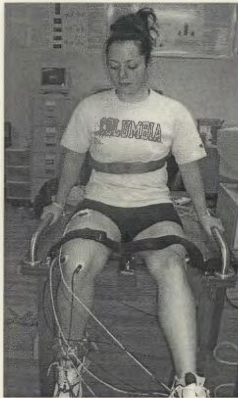
Figure 1 Quadriceps MVC set-up
